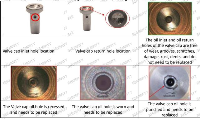
▲ The wear of the top oil return hole causes the oil return to be too large and the leaking injector cannot inject oil
